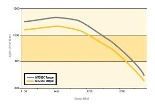
Unmatched torque rise gives the MT700C Series tractors more available power than any tractor in its class. With 52% PT0 torque rise, 42% engine torque rise, and 8% engine power growth, the MT700C series tractor can handle any application from seeding and tillage to pulling a grain cart.
