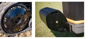
Proper ballasting is essential for peak performance, whether you're running on tracks or tires. Challenger offers everything you need to balance the load for maximum traction and fuel efficiency. Options include a full rack of front suitcase weights, as well as idler wheel weights, which, when combined, take an MT700C model up to an industry leading 36,000 pounds (16,329 kg), for maximum traction.
