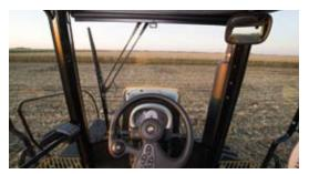
The rear ROPS cab posts are also placed in-line with your shoulders for an unobstructed view of wide, trailed implements. Meanwhile, large side mirrors and a wide-angle inside mirror let you keep an eye on equipment without the need to twist around. Electronically remote-controlled heated mirrors are optional for a clear view in all weather conditions.
