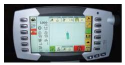
All functions of the AUTO-GUIDE<sup>2</sup> system are managed through the new TMC display. Naturally, AUTO-GUIDE<sup>2</sup> is disengaged as soon as you manually turn the wheel, whether it's at the end row or the middle of the field.
