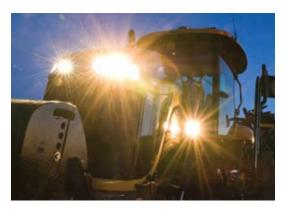
by replacing four of the eight halogen lights on the standard lighting package (two on the front and two on the rear) with HID Xenon lights.
