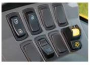
A new A/B engine speed switch on the TMC allows the operator to preset two memory settings for consistent engine speed during field operations and/or headland turns. TMC display
