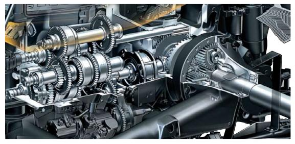
It takes a special transmission for a track tractor. The Catbuilt 16F X 4R electronically controlled powershift used in the MT700C Series was extensively tested in tough, real-world situations like yours before it was ever released to production. Since then, it's been proven reliable in hundreds of thousands of hours of field use.
