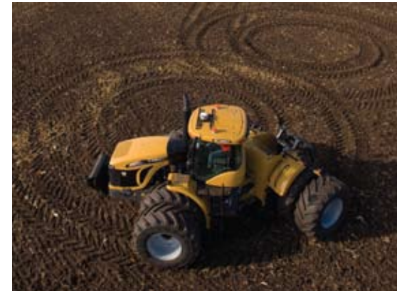
A 42-degree turn angle provides the shortest articulated turning radius in the industry allowing for tight maneuvers on headlands and corner.
