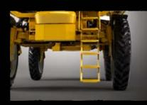
The newly engineered front entry on the RoGator starts with a step that's just about a foot off the ground and is properly angled to minimize fatigue and maximize productivity.
