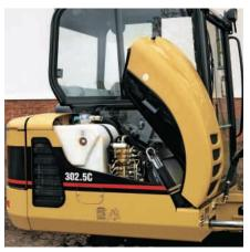
**Lift Up Side Cover.** Access to the implement valve and hydraulic tank is convenient through a lift up side cover.
