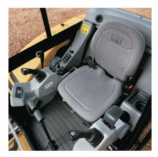
**Operator Station**. The large, spacious cab offers superior leg room, air circulation and an expansive viewing area, with flat glass throughout, for easy and inexpensive replacement.
