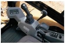
Low Effort Controls. Ergonomic, low effort controls offer greater operator comfort for increased productivity. Dozer lever mounted, two-speed travel control provides easy operation and increases foot room.
