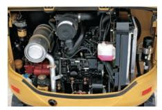
Service Access. Large, swing-out rear doors allow access to major components and service points within the engine enclosure, including:
