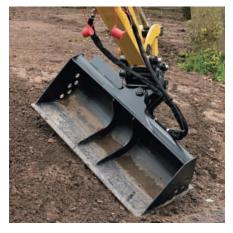
**Bucket Angle.** High rotation bucket angle combines good spoil retention and flat back trench characteristics.
