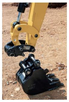
**Mechanical Quick Coupler.** The Cat Quick Coupler makes tool changes fast and easy. Maximizing performance and compatible with all standard work tools.
