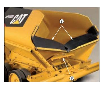
**Precise Mix Delivery.** The material delivery system provides precise mix delivery with minimal operator monitoring. The left and right conveyors in addition to the left and right augers are controlled independently.
