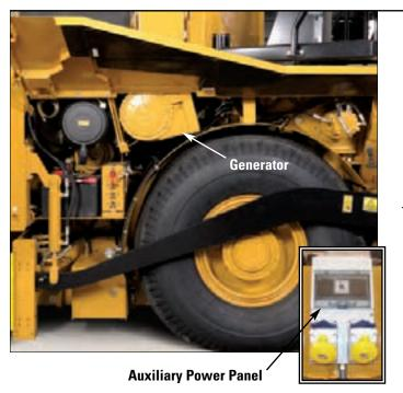
**Industrial, Single-Phase A.C. Generator.** The tractor-mounted generator provides 25 kW of power at 60 Hz for the electric screed heat and the auxiliary power panel. Circuit breaker protection, internal electronic voltage regulation and a dual bearing design provide reliability.
