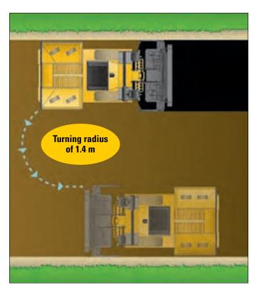
**Excellent Mobility.** The sharp turning radius and high propel speeds allow the paver to move quickly around the job site.
