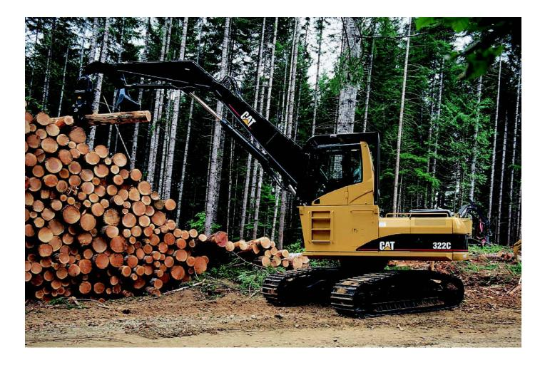
**Heel-Boom Grapples.** Factory-installed and supported heel-boom grapples are matched to the factory logging fronts to increase production and reliability. **Cab Riser**. Every forest machine is equipped with a cab riser, which helps increase operator effectiveness. Standard hydraulic tilt simplifies transportation to meet shipping height requirements. the General Forestry Machines are built with the 457 mm (18 in) riser. The Log Loader Machines are built with the 1219 mm (48 in) riser.
