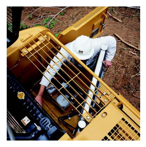
**Diagnostics and Monitoring.** The 322C FM is equipped with  $S \cdot O \cdot S^{SM}$  sampling ports and hydraulic test ports for the hydraulic system, engine oil and for coolant. A test connection for the Electronic Technician (ET) is located behind the cab.
