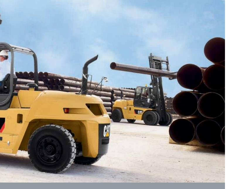
**Optimized Visibility** Narrow mast channels and an open overhead guard help improve operator visibility to the load and work area. Standard work lights illuminate your
