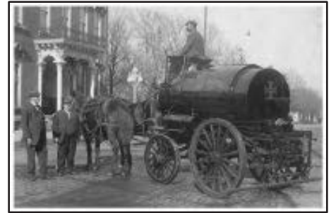
In 1910 Etnyre launched the Road Oiler, which gave contractors a way to quickly and evenly spread oil, tar or asphalt across the roadways. The unit included a wheel driven (sprocket and chain) pump and a spray bar for proper product dispersion.
