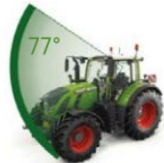
The curved windscreen of the VisioPlus cab offers a 77° viewing angle.
