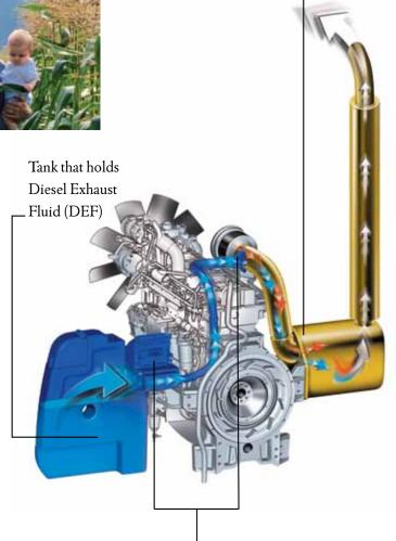
The pump and injection system unit reacts to the emissions output of the engine by continuously varying the amount of DEF added to the exhaust stream—effectively maintaining control of emissions released into the environment.
