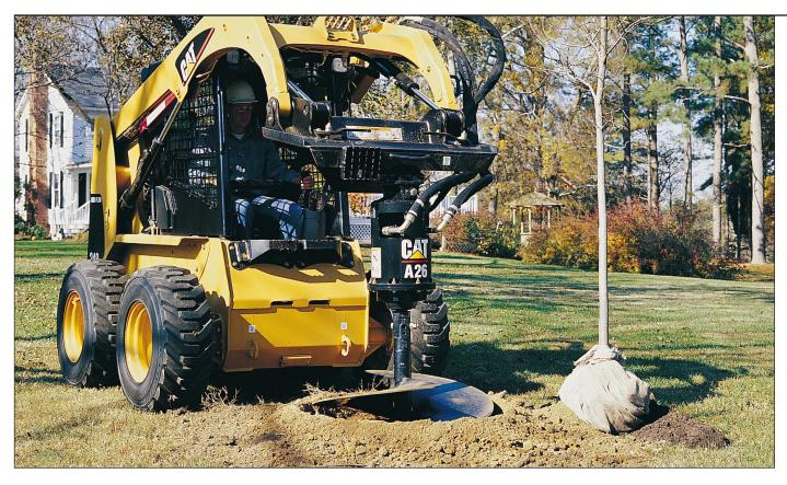
Caterpillar® Augers are used for drilling holes for footings, fencing, signs, trees and shrubs in construction, agricultural and landscaping applications. They have been designed with the right balance of speed and torque for maximum productivity in a broad range of soil types. The right amount of speed is necessary to efficiently move material up the auger bit and out of the hole. Optimal torque is required to prevent stalling when drilling in tough conditions.
