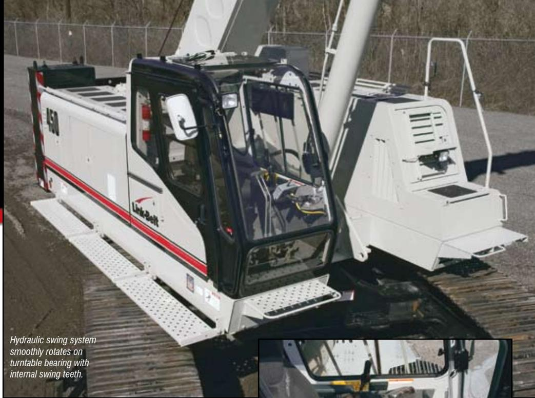
Hydraulic swing system smoothly rotates on turntable bearing with internal swing teeth.
