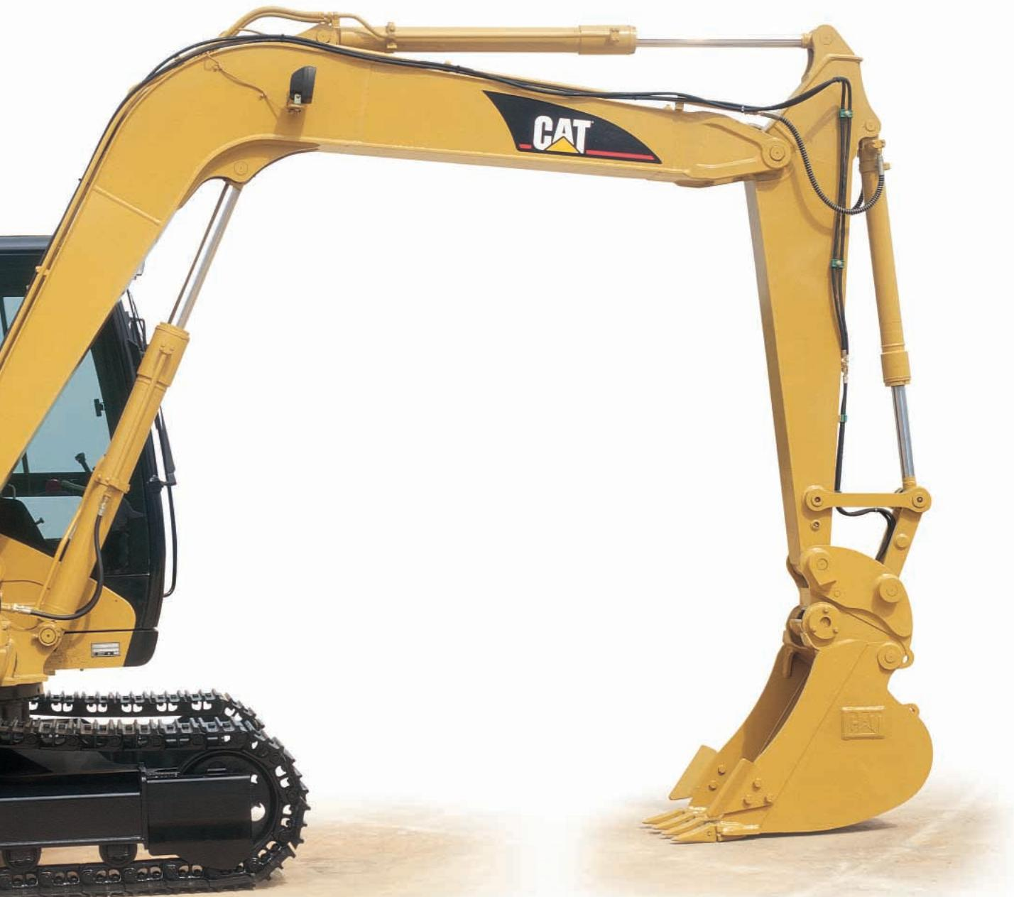
\*307C is shown with the Caterpillar Pin Grabber Plus hydraulic quick coupler and dealer-installed actuation line.
