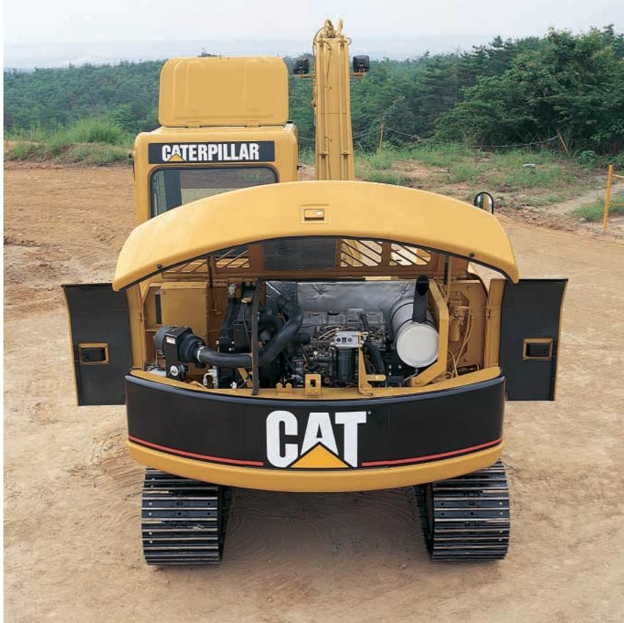
**4M40-E1 Engine.** The Mitsubishi Motors Corporation (MMC) 4M40-E1 Engine offers improved thermal efficiency with low fuel consumption and reduced low engine sound levels and vibration.
