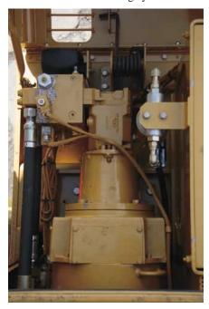
**Generator Set.** An optional 20 kW generator set can power magnets up to 66" (1.68 m) in diameter.
