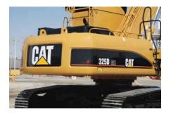
Heavy Duty Upper Frame. The upper frame is specifically designed for the scrap and material handling applications. It is built of higher strength material and thicker steel sections to handle increased swing loads from the longer front and heavier counterweights used in material handling.
