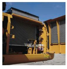
**Cooling System.** External debris filters allow easy access for cleaning. This prevents clogging from dirt and dust coming into the cooling system. The optional automatic reversing fan purges dirt and dust from cooling system.
