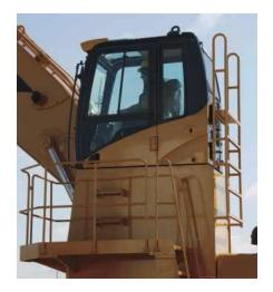
**Fixed Cab Riser.** CAT® designed and built, 6'5" (1.95 m) manual tilt cab riser provides for operating height with excellent visibility for loading and unloading processing equipment, trucks, and rail cars. Access to the cab is provided by a ladder leading up to the platform extending around the cab riser. This platform will allow for windshield cleaning. The cab riser can be manually tilted forward 90 degrees for shipping.
