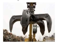
**Orange Peel Grapples.** The .75 yd<sup>3</sup> and the 1.25 yd<sup>3</sup> Orange Peel Grapples are available attachments.
