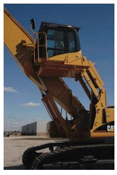
**Hydraulic Cab Riser.** Optional hydraulic cab riser provides up to 8'6" (2.6 m) of additional operating height. There is easy access to the cab platform provided by handrails attached to the riser.
