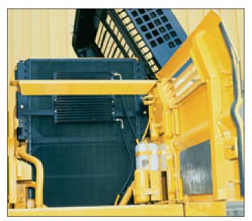
Easy clean-out engine and hydraulic cooling cores are mounted side-by-side for easy clean-out when operating in debris-laden environments.
