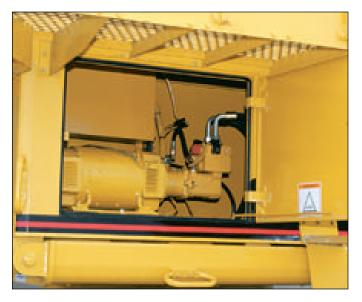
15 kW Hydraulically Driven Generator Set can power magnets up to 1477 mm (58 in) in diameter. A Baldor generator and a state-of-the-art electronic magnet controller, manufactured for Cat by Crane system, are linked to provide trouble free service. This new controller virtually eliminates traditional contactor maintenance.
