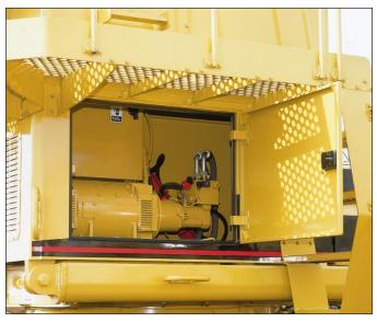
25 kW hydraulically driven generator set can power magnets up to 1829 mm (72 in) in diameter. A Caterpillar state-of-the-art electronic magnet controller and generator are linked to provide trouble free service. The new controller completely eliminates traditional contactor maintenance and it is supported and warranted through your Cat dealer.
