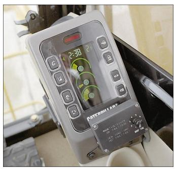
A new cab mounted magnet system monitor/control provides system information through a series of indicators, lights and a rotary selector switch, to the operator. The indicator lights provide the following information:
