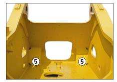
**Thicker carbody plates (2)** and increased box-section height for increased weight and load capacities.
