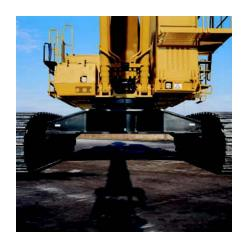
Long Square Undercarriage. Long (L) square undercarriage is standard to maximize stability and lifting capacity. The wide track gauge provides the overthe-side stability required to handle heavy loads and improve productivity, but is also retractable to provide a narrow gauge and reduced shipping width.
