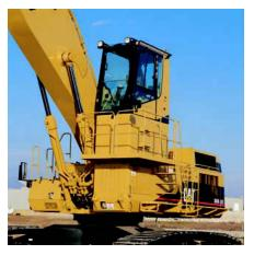
**1.9 m (6'5") Cab Riser**. Cat designed and built cab riser gets your operator to an operating height with excellent visibility for loading or unloading your processing equipment, trucks, rail cars, and barges. Access to the cab is provided by a platform which extends around the riser to allow windshield cleaning. The cab riser can also be manually tilted forward 90 degrees for shipping.
