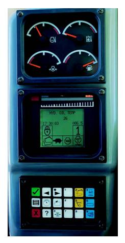
**Operator Station.** The work station is designed to be quiet and comfortable for the operator, assuring high productivity during a long work day. The Caterpillar designed electronic control system uses VIDS (Vital Information Display System) as the easy interface between the machine and the operator or the serviceman.
