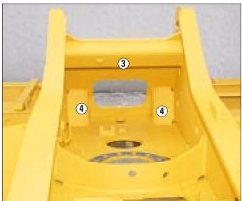
Box-section cross member (3) and box-section cylinder mounts (4) help handle increased torsional loads and payloads.
