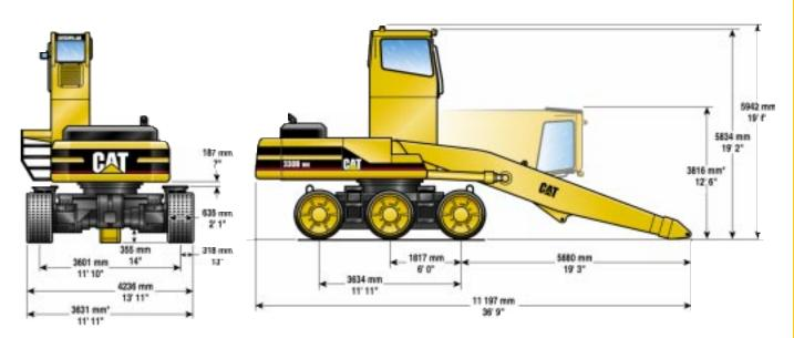
\* Shipping dimensions require removal of wheel assemblies, ladder, walkway and handrail assemblies on left-hand-side of cab riser, handrail group on right-handside of tool box and walkways on wheeled carrier.
