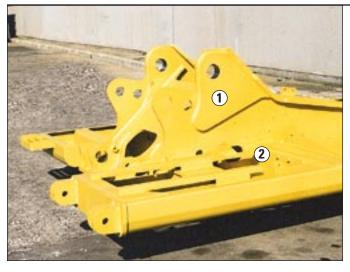
**The upper frame** is specifically designed for the scrap and material handling market. It is built of higher strength material and thicker steel sections to handle the increased swing loads developed with the longer fronts and heavier counterweights used in material handling.
