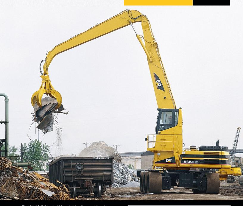
The W345B II Wheeled Material Handler combines the Caterpillar® 345B II MH base machine upper components with Caterpillar's innovative six wheeled lower to provide the scrap and material handling customer with a mobile machine, while maximizing stability for production applications.
