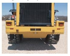
**Counterweight.** The one-piece counterweight is integrated into the 972H design and styling. This 5,849 lb (2653 kg) counterweight incorporates the rear lights into the top of the structure.
