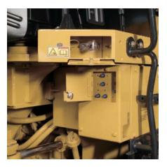
**ELECTRIC SERVICE CENTER.** Batteries, relay panel and an optional tool box are conveniently located below the left-side access platform. The engine shutdown switch is housed with the relay panel. A compartment integrated into the access platform contains the hood tilt actuation switch, master switch and optional jump-start receptacle.
