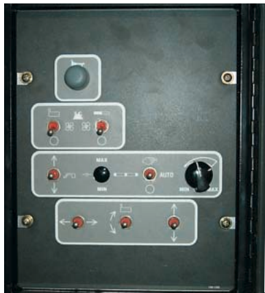
Left side main screed and extender controls
