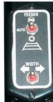
Right side main screed and extender controls
