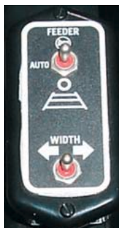
Left side main screed and extender controls
