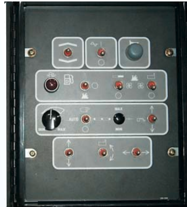
Right side main screed and extender controls
