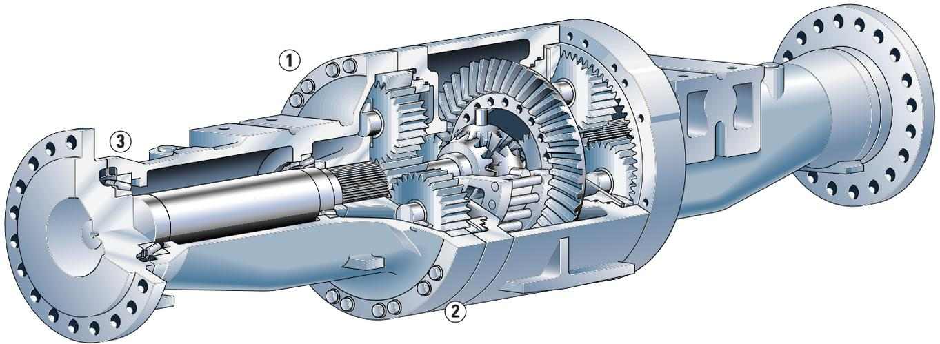
**1 Heavy-duty axles and brakes** are designed to last in all kinds of operating conditions. Planetary final drives use full-floating, bronze sleeve bearings in the planet gears. Differential components are larger and more heavy-duty than those used on the F-series machines.
