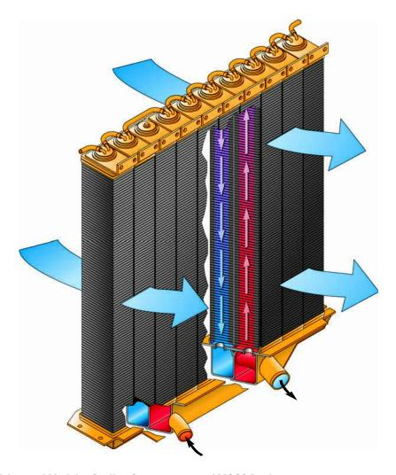
Advanced Modular Cooling System (AMOCS). Is a Caterpillar exclusive technology which improves serviceability and reduces downtime. It utilizes an exclusive two pass cooling system and increased cooling surface area to provide significantly more cooling capacity than conventional systems.
