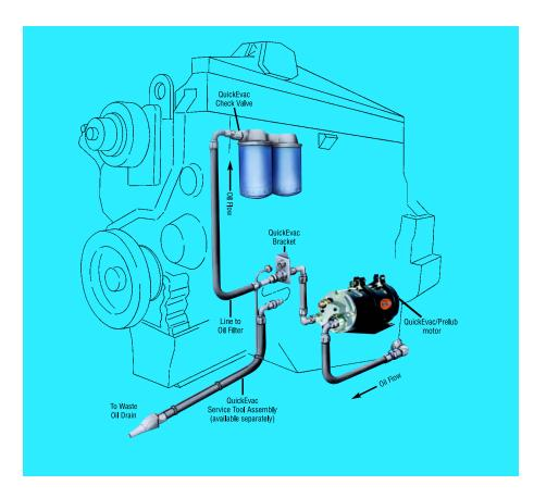
Cat QuickEvac™ System. Is an exclusive Caterpillar on-board engine oil evacuation and prelubrication system.
