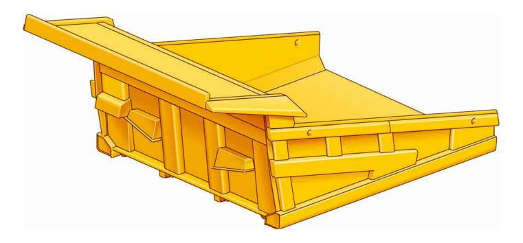
**Design.** 771D bodies are designed to handle a variety of material densities. Maximum payload is reached in three to five passes from a matched Cat loader in 1620 kg/m³ (2,700 lb/yd³) material and higher.
