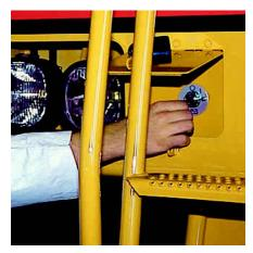
**On-Board Diagnostics.** With CEMS, provides the machine operator with a three-category warning system and quick access to stored diagnostic data.
