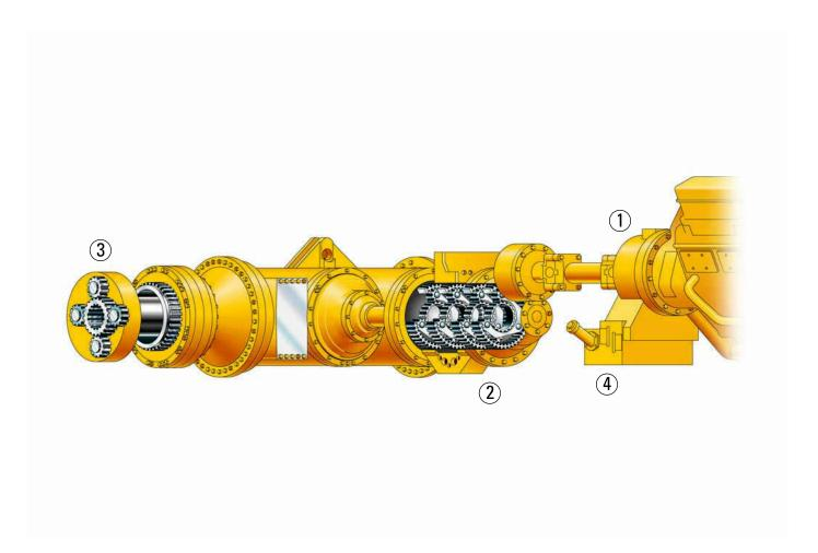
**Transmission.** The Cat six-speed, power shift transmission, matched with the direct-injection 3408E diesel engine provides constant power over a wide range of operating speeds.
