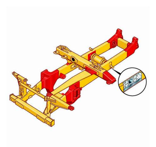
**Box-Section Design.** The 771D frame uses a box section design, incorporating 17 castings in high stress areas with deep penetrating and continuous wraparound welding. Mild steel, which provides flexibility, durability and resistance to impact loads even in cold climates is used throughout.
