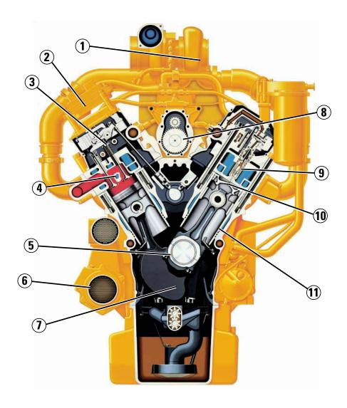
**Cat 3408E Diesel Engine.** The four-stroke design uses long power strokes for more complete fuel combustion and optimum efficiency. Large displacement and a low speed rating can help extend engine life. This engine meets U.S. Environmental Protection Agency Tier 2 emissions regulations and Stage II EU Emissions Directive 97/68/EC.
