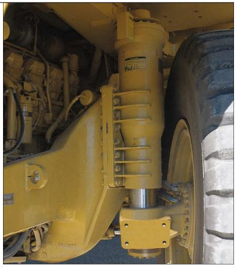
**Durable, simple design** utilizing large diameter bore and low pressure nitrogen/oil. This design provides long life and low operating and rebuild cost.
