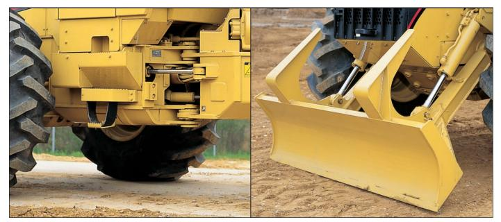
**New wider hitch pin spread** significantly reduces horizontal loading on hinge pins and hinge pin bearings for improved pin and bearing life.
