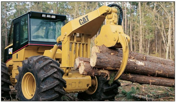
**Load sensing hydraulics** utilize a load sensing, variable displacement pump and pressure compensating system, which continually monitors braking, steering, and grapple hydraulic power requirements.
