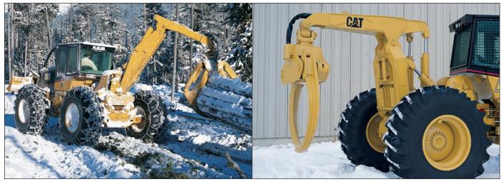
For the ultimate in skidder flexibility, the 525 is available with installed swingboom and grapple. With excellent balance and outstanding visibility, the 525 with swingboom is an ideal tool for very rough or soft underfoot terrain, thinnings, and select cuts. It also provides superior pre-bunching capabilities.
