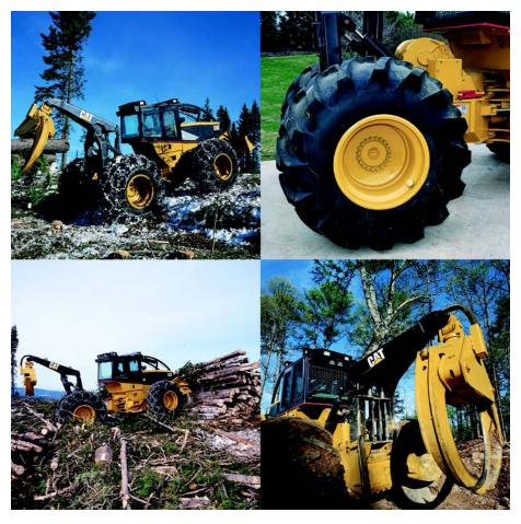
**Balance.** Long front and rear frames and a low center of mass create excellent skidder balance. The powerful mechanically driven, heavy-duty winch provides outstanding grapple or cable skidder performance.
