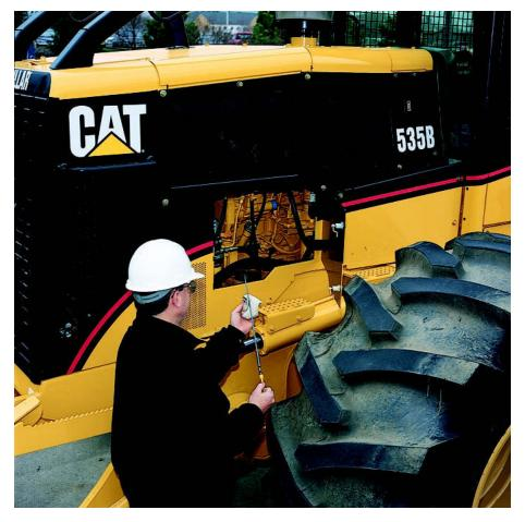
**Built-in Servicing Ease.** Caterpillar uses intelligent engineering to make regular maintenance procedures quick and simple. Easy access to daily service points increases the likelihood that maintenance will be done, extending machine service life and lowering overall operating costs. In addition, less service time means more working time and greater productivity.
