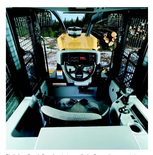
**Single-lever Grapple Control.** A single four-function lever controls all grapple and tong functions for simplified operation and reduced operator effort.
