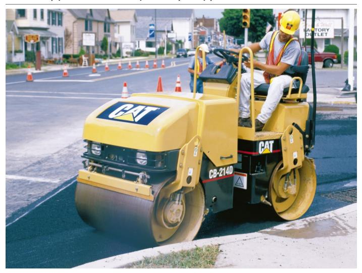
The CB-214D, CB-224D and CB-225D are versatile machines that can be used as the only compactor on small sized jobs or on larger jobs as a support roller for high-production compactors. As a support roller, they work well for turning lanes, crossovers, shoulders and other similar sized jobs.
