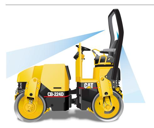
**Excellent forward visibility** allows the operator to see objects 0,58 m (1.9') high and 1 m (3.3') in front of the machine.
