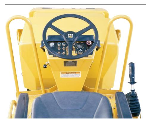
**Single-lever control** provides simplified operation, making the machines a perfect fit for inexperienced operators.
