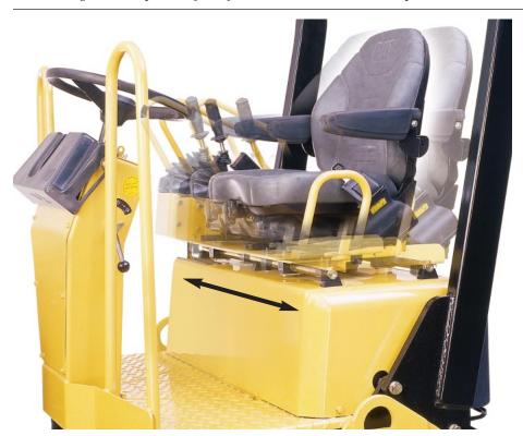
**Seat slides from side to side** and locks into three positions – right, center and left.
