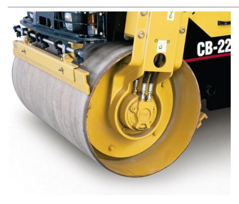
**Specially designed drum edges** help eliminate marks on deep lifts or when turning. Note: CB-214D and CB-224D can be equipped with optional Non-Machined Drum Edges that have a square profile instead of the standard design.
