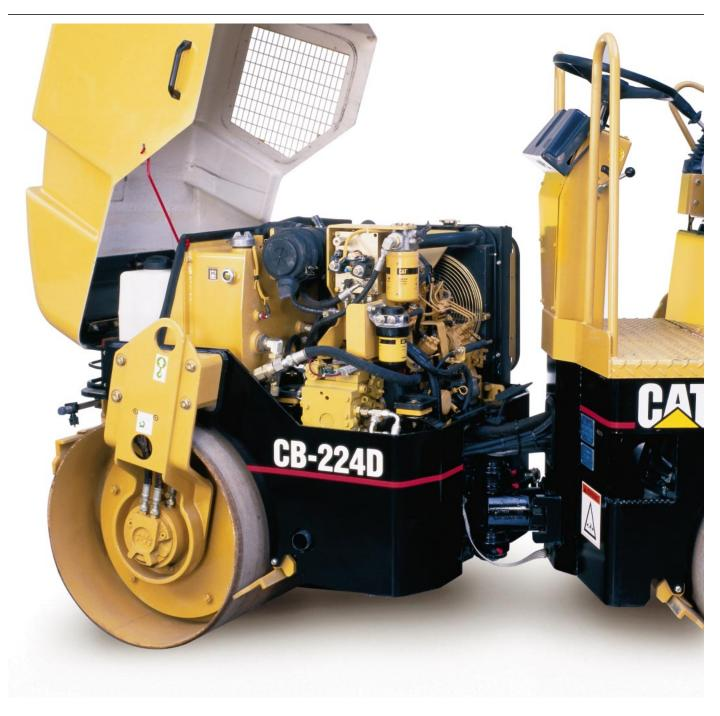
**Fiberglass engine enclosure** pivots upward and locks open with a prop rod.
