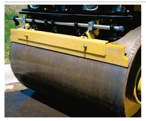
**Constant or intermittent spray capabilities** provide extended operation between refills.
