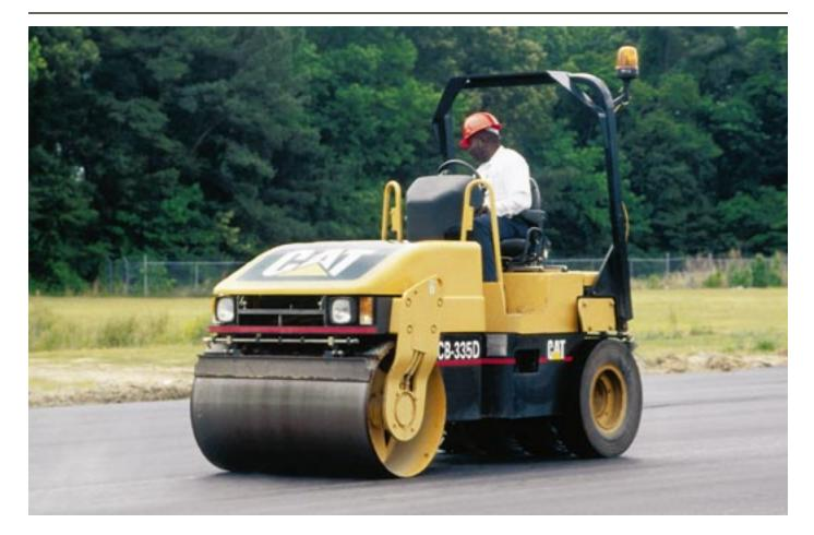
The CB-334D and CB-335D are versatile machines that can be used as the only compactor on small to intermediate sized jobs or on larger jobs in conjunction with high-production models.
