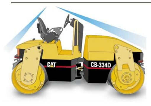
**Excellent forward visibility** allows the operator to see objects 0,6 m (2') high and 1 m (3.3') in front of the machine.
