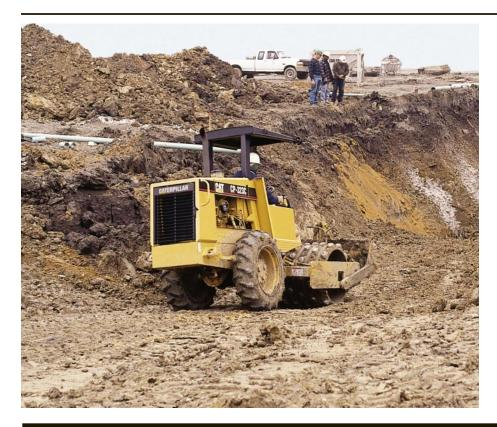
**Narrow machine width** of 1393 mm (54.8") is ideal for working in trench applications or limited space job sites.
