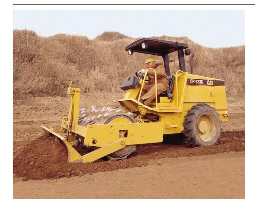
**Single lever blade control** located to the right of the operator's seat for simple and convenient operation.
