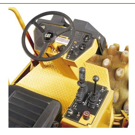
**Single lever control** for propel and vibratory On/Off provides simple, one-handed and low effort operation.
