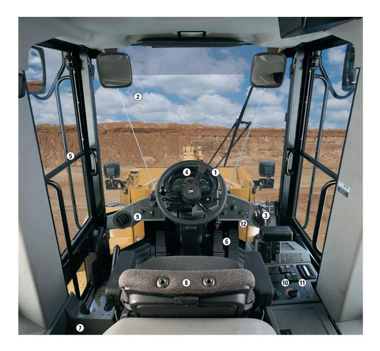
**1 Steering.** Low effort hand metering unit steering. Tilt steering column helps fit the wheel to the operator. Load sensing steering directs power through the steering system only when needed. When not steering, more engine power is available to generate rimpull, breakout and lift forces.
