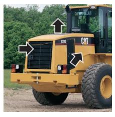
**Reverse Flow.** Air enters through the rear grill and exits out the top opening and side hood doors. Rear air flow picks up less debris from the ground, reducing plugging.
