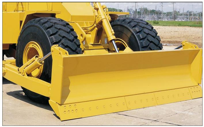
**Does light production** including dozing and spreads fill, backfills, stockpiles, charges hoppers, and cleans up around shovels and trucks. **Two levers at operator's right** control dozer lift/tilt and tip.
