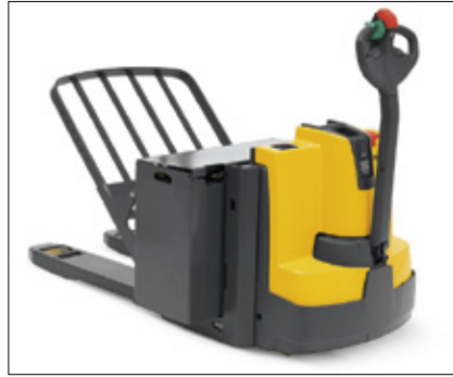
Side battery extraction on EJE 225 E.
