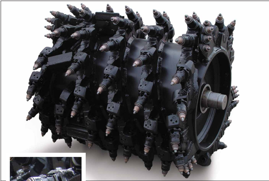
Quick release three-piece tool holder.
