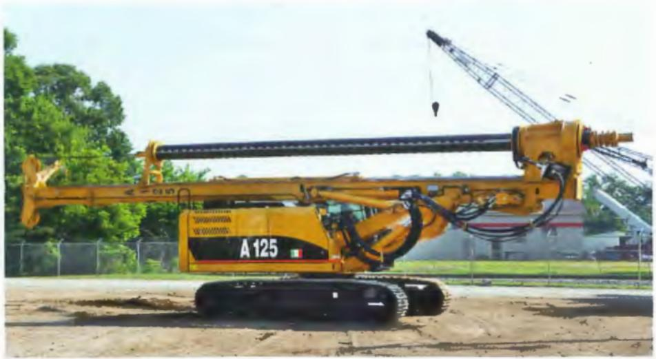
Kelly Tractor Co. recently introduced the new A125 drill rig to North America. Built in collaboration with IMT and Caterpillar OEM Solutions Group, the pioneering redesign enables the Tier 4 rig to lay flat for complete single load transport.
