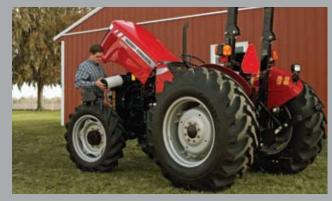
Most daily service items, such as engine oil check, can be done without opening the hood. For other maintenance, the gas assisted, single-piece steel hood opens widely for easy access.
