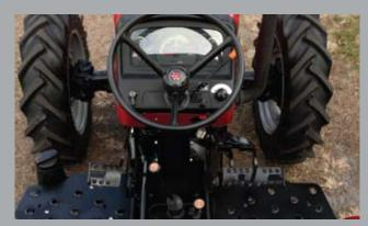
An economical 8x2 constant mesh transmission with live PTO provides a simple and reliable powertrain to handle daily chores on the farm. The optional 8x8 SynchroShuttle transmission with independent PTO gives new meaning to comfort and convenience by allowing the tractor to shift gears on the go and change direction without having to stop completely.
