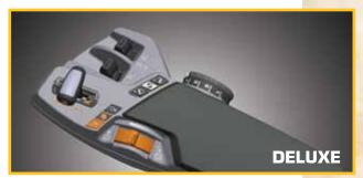
Short control armrest features T-handle transmission and fingertip-controls for hydraulic remotes, three-point hitch, engine speed and headland, throttle and power management.
