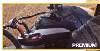
Multipad armrest with Multipad joystick for thumb and fingertip control of forward/reverse shuttling, PTO, programmable hydraulic function, engine and cruise speeds.
