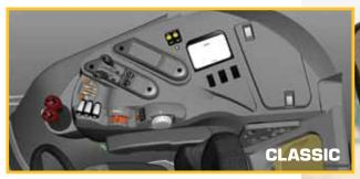
Familiar layout ergonomically places T-handle transmission level and hydraulic controls within easy reach on ride-side console alongside PTO and three-point hitch controls.
