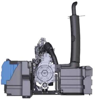
e3 is a post-combustion, after-treatment process that takes place in the exhaust system, never interfering with the performance of the engine itself.
