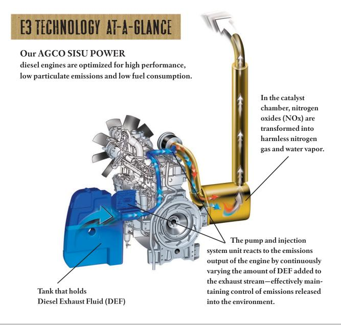
As simple as it is effective, our e3 version of SCR technology treats the down-stream exhaust with Diesel Exhaust Fluid (DEF), which breaks down harmlessly into nitrogen and water vapor. Believe it or not, the e3 process, along with electronic engine management, actually allows our AGCO SISU POWER $^{\text{m}}$  diesel engines to run better, stay cooler and last longer.
