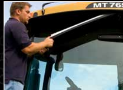
The cab air filter is easy to access and clean out.
