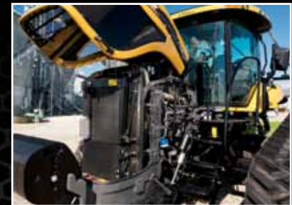
By simply tilting up the hood, you have easy access to all engine service points and cooling package cleanout.
