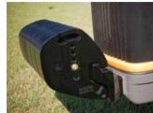
Proper ballasting is essential for peak performance, whether you're running on tracks or tires. Challenger offers everything you need to balance the load for maximum traction and fuel efficiency. Options include a full rack of front suitcase weights, as well as idler wheel weights, which, when combined, take an MT700C model up to an industry leading 36,000 pounds (16,329 kg), for maximum traction.
