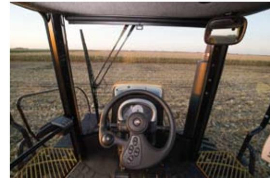
In addition to 67.5 square feet (6.2 m<sup>2</sup>) of usable glass area, Challenger® MT800C/MT900C Series tractors feature a short, sloping hood that provides an unobstructed, panoramic view of the field.
