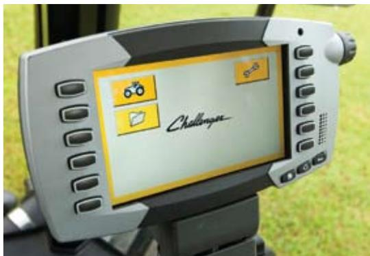
Comprised of a color screen, 12 soft keys and a rotary dial the ISOBUS compliant TMC display allows the operator to monitor all tractor, engine, and transmission functions; check and adjust hydraulic flow settings; keep track of service intervals; operate the AUTO-GUIDE<sup>2</sup> system, and collect valuable data that can later
