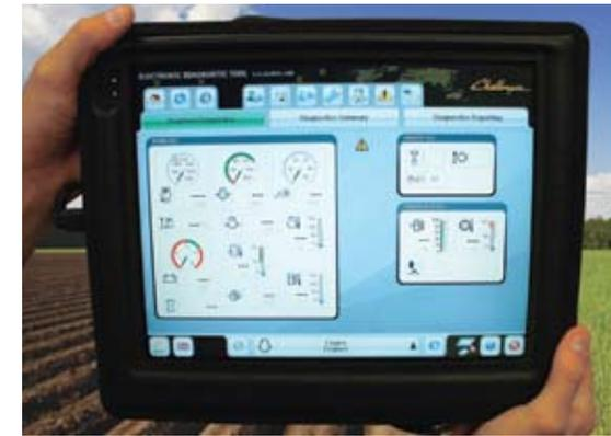
Downtime never comes at a convenient time! Fortunately, it doesn't take long to locate a problem, thanks to our new ISOBUS technology. Since every component on the tractor communicates in the same language, a service technician need only plug in a portable, hand-held unit that performs diagnostics and displays results in a matter of seconds.
