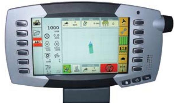
All functions of the AUTO-GUIDE<sup>2</sup> system are managed through the new TMC display. Naturally, AUTO-GUIDE<sup>2</sup> is disengaged as soon as you manually turn the wheel, whether it's at the end row or the middle of the field.
