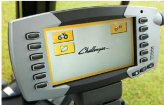
The all new TMC display found in the MT700C Series is comprised of a color screen, 12 re-programmable soft keys, and a rotary dial. This ISOBUS compliant unit allows the operator to monitor and manage all tractor functions, track service intervals, manage the AUTO-GUIDE<sup>2</sup> system, and collect valuable data for total farm management...all from one convenient location.
