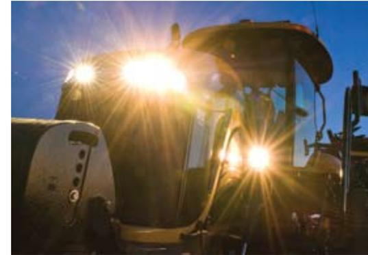
by replacing four of the eight halogen lights on the standard lighting package (two on the front and two on the rear) with HID Xenon lights.
