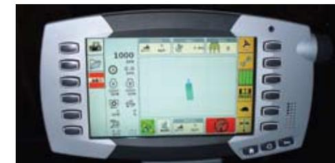
All functions of the AUTO-GUIDE<sup>2</sup> system are managed through the new TMC display. Naturally, AUTO-GUIDE<sup>2</sup> is disengaged as soon as you manually turn the wheel, whether it's at the end row or the middle of the field.
