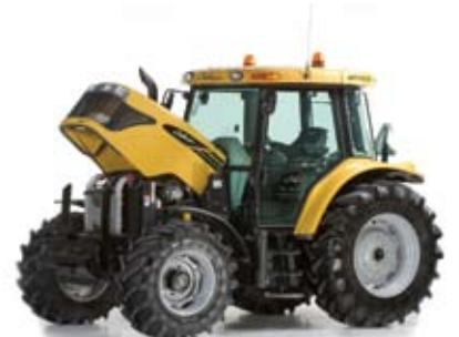
The redesigned hood lifts at the front for quick, easy access to the cooling system and front of the engine.
