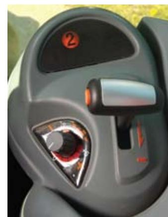
The Auto-Power IV transmission has all powershift and range shift controls on one pivoting T-handle lever.
