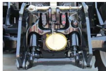
A restyled front casting on the new 100-horsepower (75 kW) MT475B allows the option of a front-mounted PTO, as well as the factory-installed 3-point hitch and hydraulic remotes available on all models.
