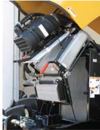
The new expanding cooling system on the MT475B combined with a cassette-type air filter that can be replaced quickly, makes service even less time-consuming.
