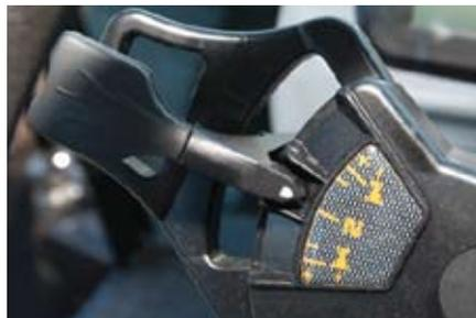
The multi-function power shuttle puts directional change, powershifts and transmission declutching right at your fingertips.
