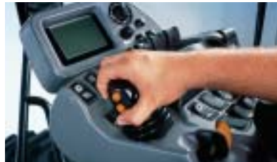
Shift and Power Management buttons are placed close at hand for maximum productivity. In park position, steering is locked preventing inadvertent machine movements.
