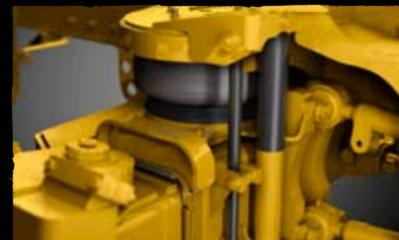
An onboard system automatically adjusts the pressure in the air spring suspension to deliver a smooth, level ride for optimal comfort and minimal fatigue.
