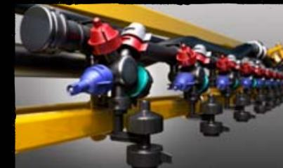
Protected spray nozzles ensure that even if a boom hits the ground, the nozzle stays put – saving you the time and hassle of machine repair while reducing the risk of spill or misapplication.
