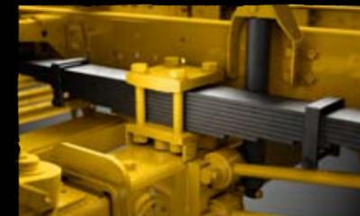
Our heritage models come equipped with a leaf spring suspension that helps even out the ride over challenging terrain while maintaining responsive handling and control.
