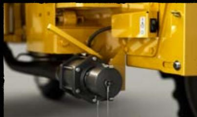
New front reload option for chemicals reduces refill time without folding the boom.
