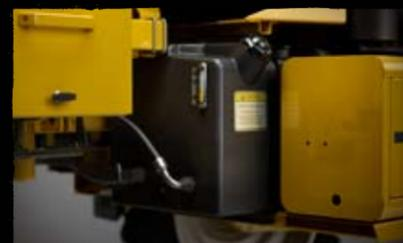
A large 60-gallon (227 L) hydraulic reservoir keeps fluid cooler and delivers enough capacity to handle auxiliary hydraulics.
