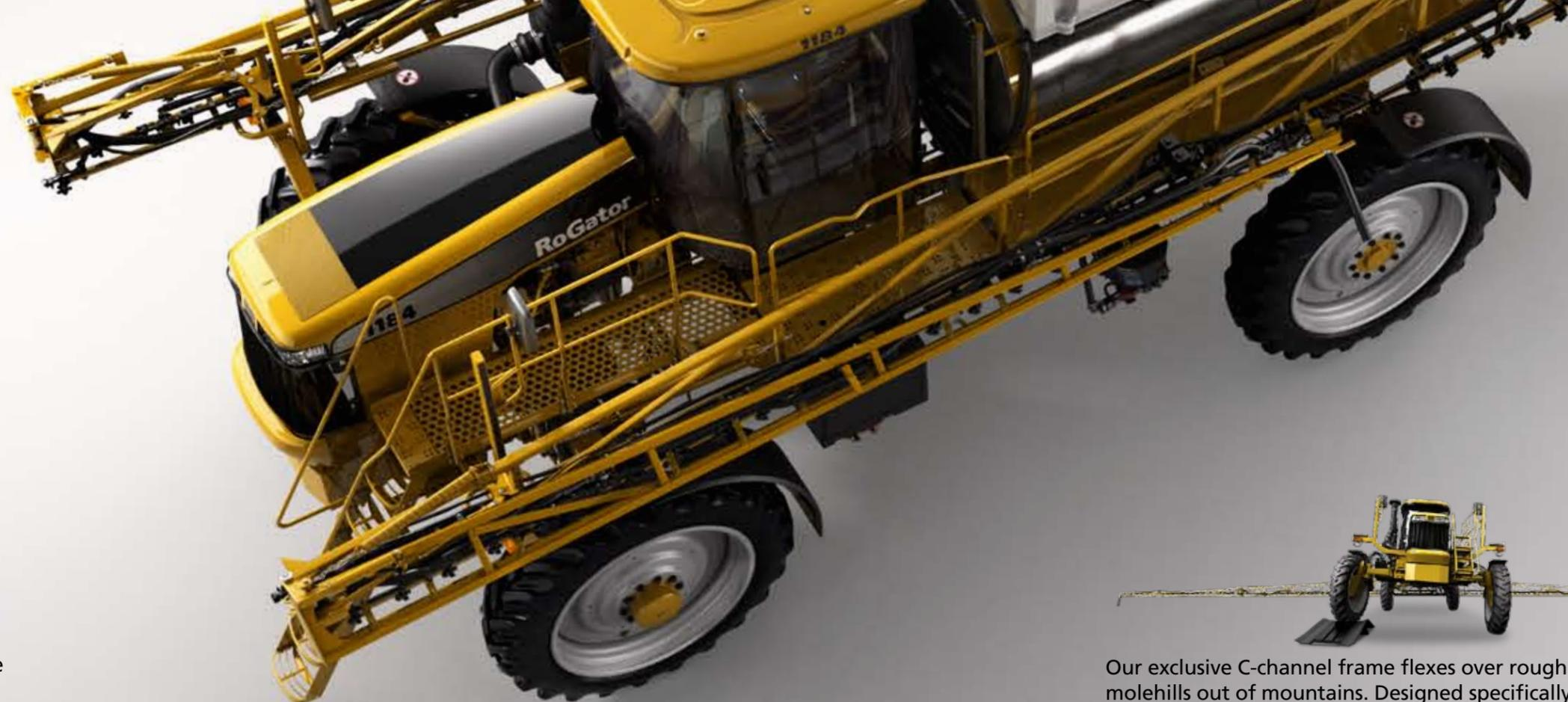
Tight turns are no match for RoGator thanks to an incredible 23 ft. (7 m) turning radius that shrinks to an amazing 13.5 ft. (4.1 m) when you add the Gator Trak four-wheeled steering option. You'll cover more acres in less time with greater accuracy.
