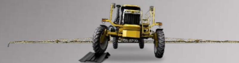
Our exclusive C-channel frame flexes over rough terrain – making molehills out of mountains. Designed specifically for spraying applications, the frame maintains strength and flexibility to withstand tough demands, while reducing the risk of cracking for lower maintenance costs and less downtime.
