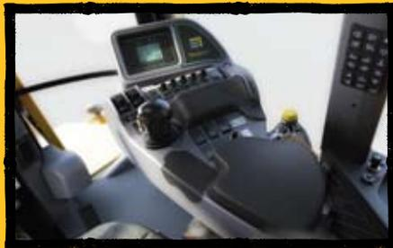
All application functions are in the right-hand console adjacent to the operator's seat. The master apply switch, gear selection, boom wing up/down, foam marker and individual boom control are within reach of your fingertips.
