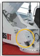
Allows operator to check eight (8) pressures and grease four (4) different points from one centralized location on the upper frame. Boom foot pins, head machinery sheaves, and cab tilt cylinder are also greaseless
