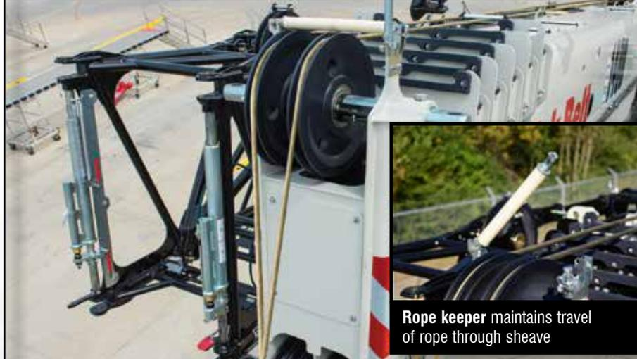
Rope keeper maintains travel of rope through sheave
