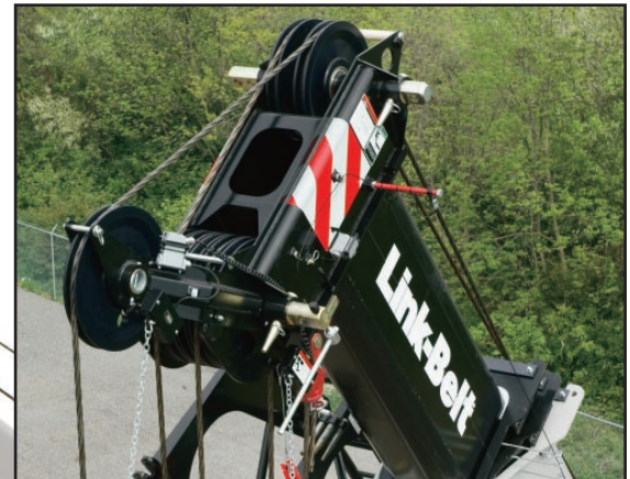
Optional hoist drum cable follower and optional third wrap indicators
