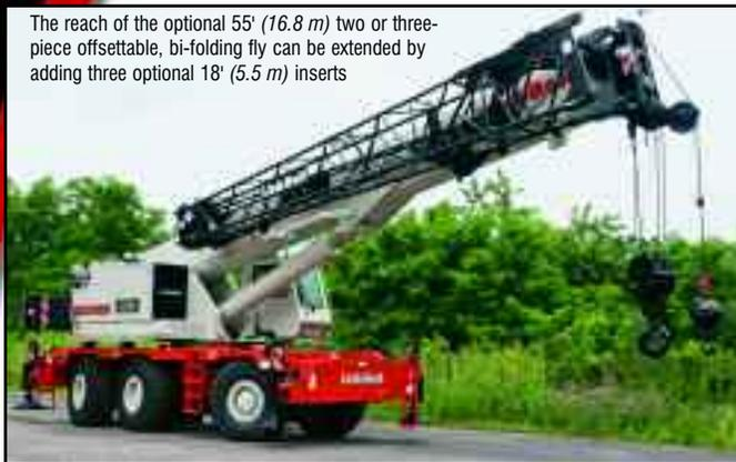
The reach of the optional 55' (16.8 m) two or three-piece offsettable, bi-folding fly can be extended by adding three optional 18' (5.5 m) inserts
