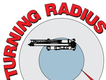
Because of the innovative 6x6 hydrostatic drive/steer on each wheel, the turning radius of the 28' 10" (9.1 m) long carrier is a remarkable 21' 10" (6.6 m).
